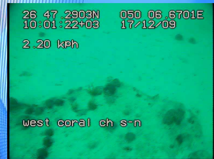
Towed video with GPS overlay is used to cover the impacted area quickly and provide a useful overview plus comparison footage of adjacent un-impacted reef.
