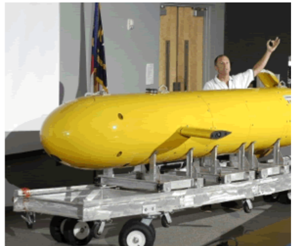
Figure 4: Major equipment to be used on 2006 cruise: Left — Phantom SII ROV on deck of Liberty Star ; Right — Eagle Ray AUV with multibeam echosounder.
