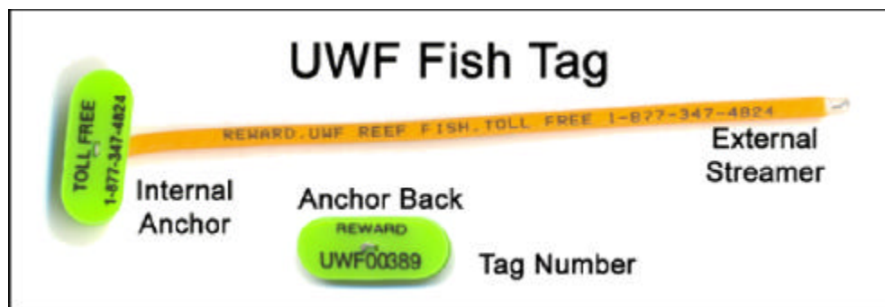
Figure 6. Digital images of an internal anchor tag used in this study. Tag length is 80 mm; anchors are 6 mm wide and 16 mm long.
