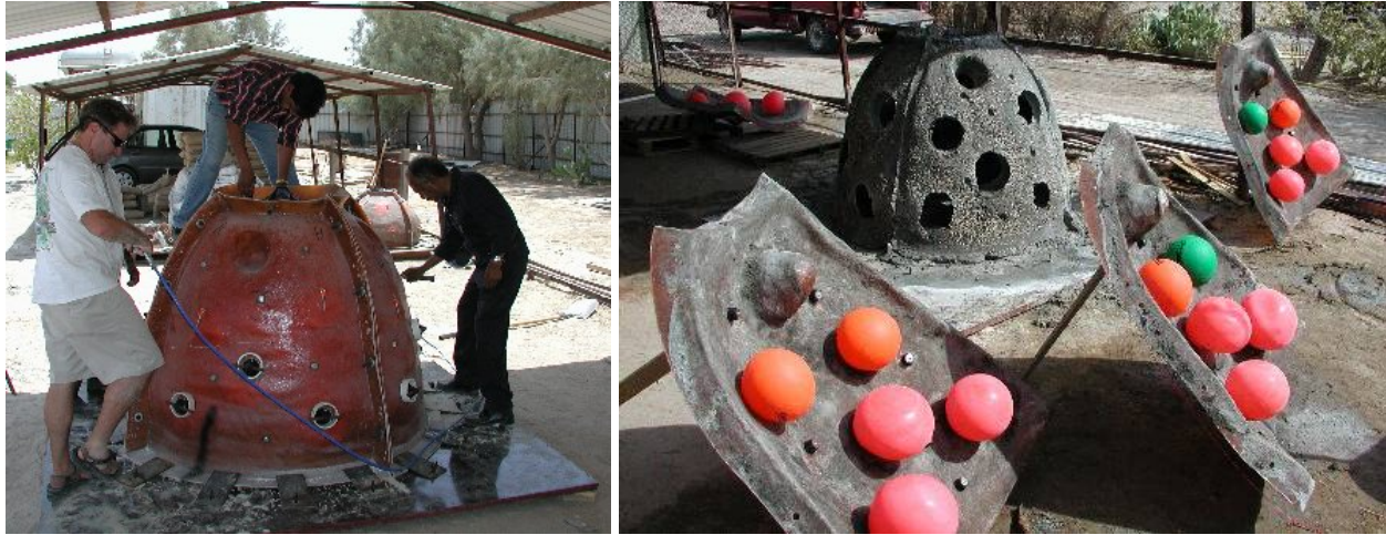
Figure 2. Traditional Reef Ball Unit Mold Fabrication
