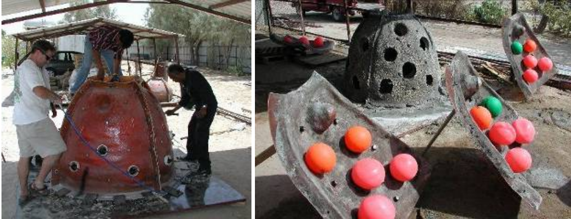
Figure 12. Traditional Reef Ball Unit Mold Fabrication
