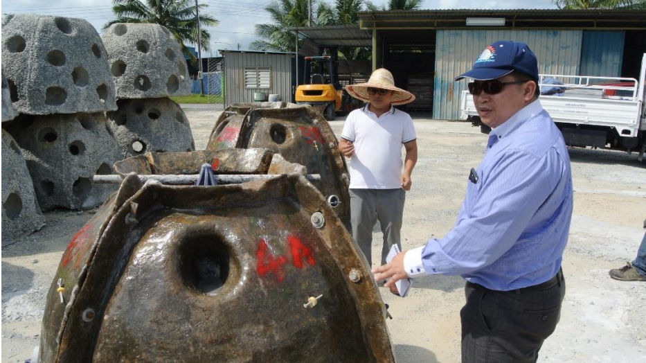
Figure 11. Reef ball mould quality inspection
