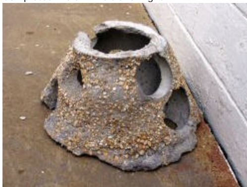
Here is the finished product! This reef ball will provide habitat for fish and other aquatic life, while providing a surface for oysters to attach and filter water. See CBF's website for more info on oyster reefs and reef balls.
