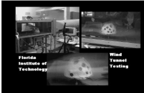
Wind tunnel demonstrating whirlpool effect of Reef Balls
